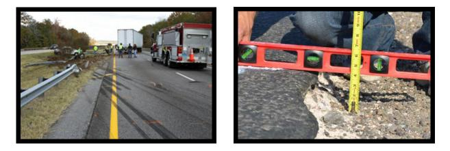
Photographs and videotapes are most useful when they incorporate a road sign or other stationary fixture or feature of the roadway or terrain for reference, and for pictures with a tighter focus, a ruler or tape measure placed near the item depicted is useful to establish scale.
