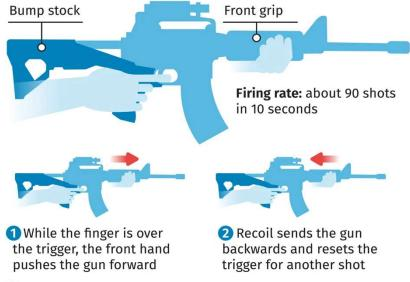
3 For as long as the front grip is pushed forwards, the process is repeated and the gun continues to fire
